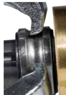
Lock on ball grooves and bearing races.
