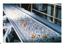
and other high-temperature materials, the material temperature does not exceed 800°C, the belt temperature does not exceed 220°C.
