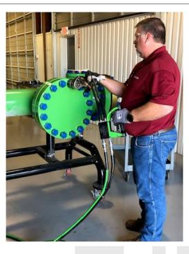
Engineered to provide operator safety whilst positioning and operating hydraulic Torque Wrenches
